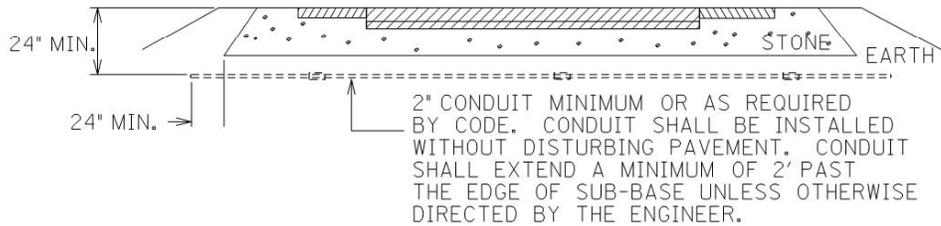
2" CONDUIT MINIMUM OR AS REQUIRED BY CODE. CONDUIT SHALL BE INSTALLED WITHOUT DISTURBING PAVEMENT. CONDUIT SHALL EXTEND A MINIMUM OF 2' PAST THE EDGE OF SUB-BASE UNLESS OTHERWISE DIRECTED BY THE ENGINEER.
