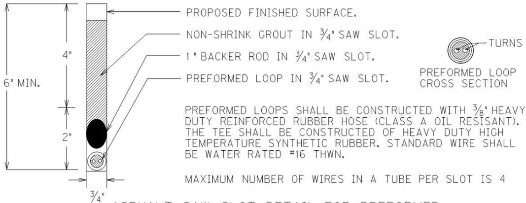
PREFORMED LOOPS SHALL BE CONSTRUCTED WITH  $\frac{3}{8}$ " HEAVY DUTY REINFORCED RUBBER HOSE (CLASS A OIL RESISTANT). THE TEE SHALL BE CONSTRUCTED OF HEAVY DUTY HIGH TEMPERATURE SYNTHETIC RUBBER. STANDARD WIRE SHALL BE WATER RATED #16 THWN.
